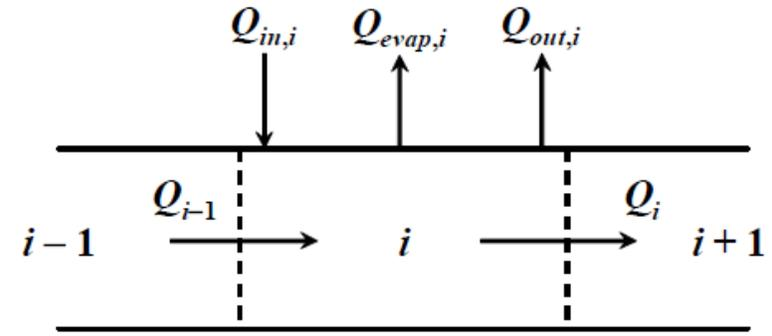
QUAL2E model assumes steady, nonuniform flow. The term steady flow refers to flow that does not vary temporally. The term nonuniform flow means that it varies spatially. For this characterization a flow balance for element  $i$  can be written as:
