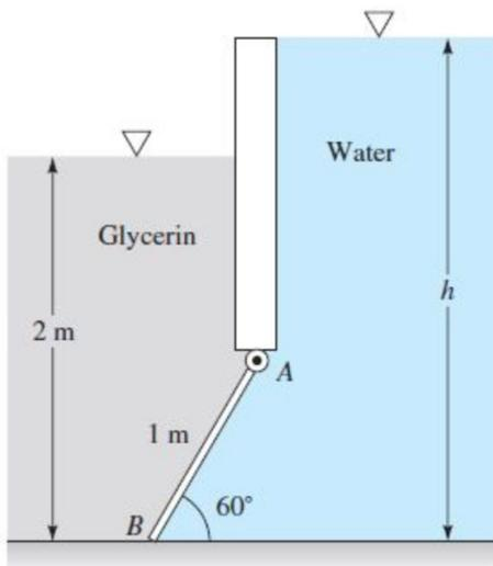
Assume AC (vertical distance of Gate AB) is equal to  $(AB)\sin\theta = (1\text{m})(\sin 60 \text{ degrees}) = 0.86666$
